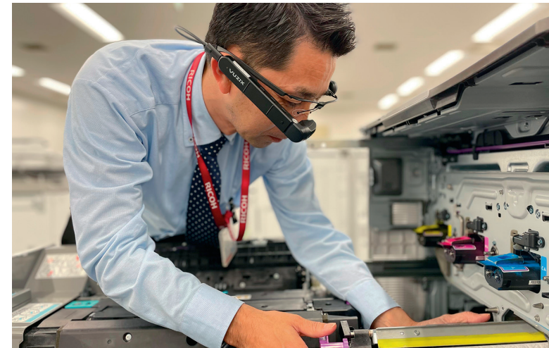
An engineer wears Vuzix M400 smart glasses at a customer facility, providing multi-function device maintenance with remote support from the branch office (posed photo)
